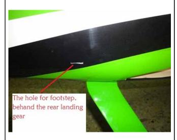
2. There is a blind nut for the footstep inside the fuselage.
