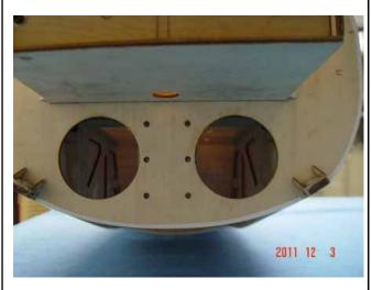
2. Mount the front landing gear to the fuselage with 6 bolts.
