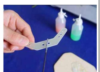
5. Slid the horn into slot slightly ,mount the locking plates in place. Wipe away excess glue with rubbing alcohol
