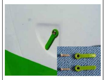
Drill a 1mm diameter hole. Then screw the bolt to fix the canopy lock.
