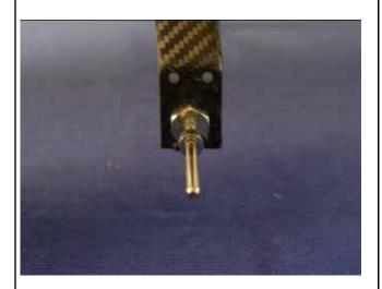
6. Install the collars and wheel in order with **a drop of Blue Loctite** on the collar set screw and ensure the wheel is free to rotate.
