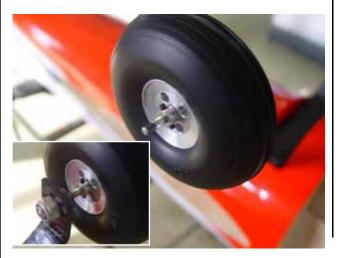
7. Drill the holes for the mounting bolts and install the blind nuts.
