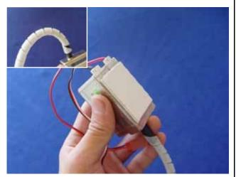
2. Position the ignition outside the engine box to allow the spark plug leads to connect the engine without excess tension .Drill for Nylon tie
