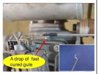
3. Determine where the throttle servo mounting tray is going to be mounted on the engine box to get the straight and precise throttle linkage connection then make a mark
