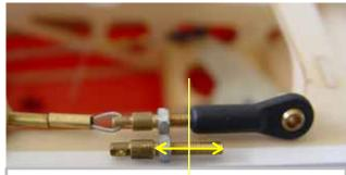
NOTICE: The coupler is best to thread half way into ball link for further tightening next
