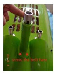
3. Screw other bolts on the back of the landing gear covering.
