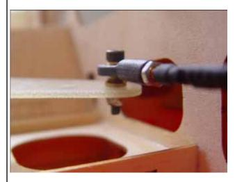
10. Turn off the radio now. Reinstall the ball link (Don't pull strongly to hurt the rudder or back to step 7 for readjustment )you can find a helper and do that at certain deflection with supporting the bottom of the rudder.
