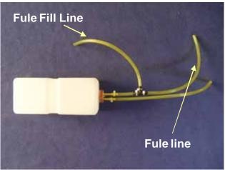
Fule tank and fule dot have been installed. Just tighten the velcro ties
