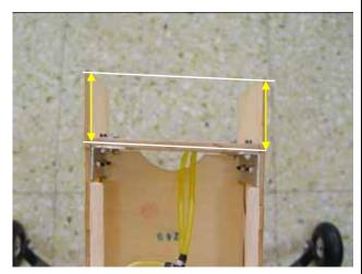
Note: There are both right thrust line and down thrust line marked on the engine box.
