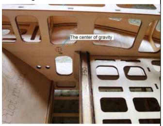
Your balance at the CG will determine batteries final mounting location.
