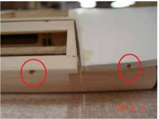
2. Put some glue on the black tip of the antennas. Then insert the antennas into the hole.
