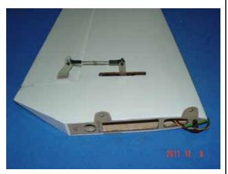
4. Lock the connector with the provided safety clip against vibration and loosened tension as shown
