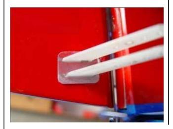
Make sure the horn line up with ground and align the both side before epoxy has cured`
