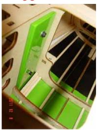
3, Install the aluminum connecting angle between two side landing gear as shown
