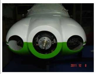
1. Measure the length of the engine (from the firewall to the prop thrust washer), the cowl and the engine box for the proper distance allowing 1/4"to 1/2" from the edge of the cowl .Then mark the location
