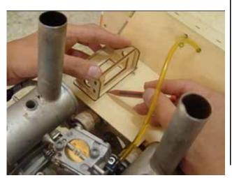
4. Epoxy the mounting tray in place and secure with self-tapping screws
