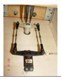
7. Adjust the rod length to make the front wheel in the middle place.
