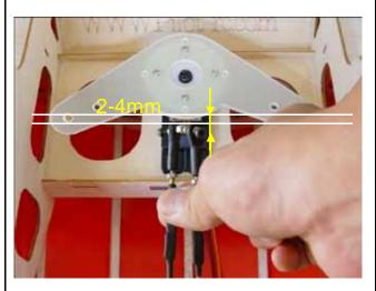
8. Shrink the heat shrinking tube on the brass tube
