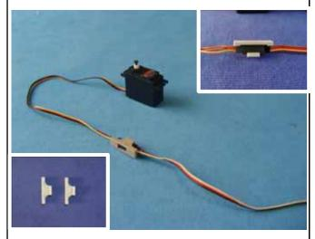
3. Cut out the cover for servo location carefully .Tape the lead to pull-string tightly. In order to ensure the servo wire can be pulled out without hanging up inside wing
