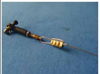
7. Thread the coupler in 2-4 mm (according the bolt holes center). Ensure the same length of cables and tension
