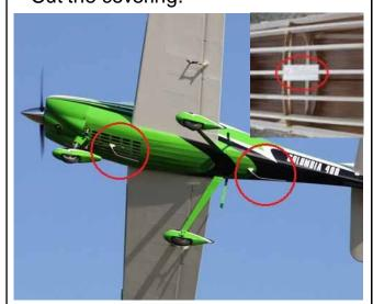
2.Glue the accessories on the bottom of the fuselage.
