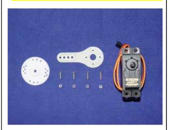
1. Turn on your transmitter and plug the servo into receiver. Ensure every channel is neutral
