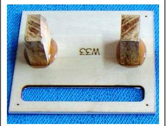
7. Use 1mm bit to drill the mounting holes. Then screw four bolts to fix the servo to the servo mounting.
