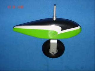
3. Screw two side bolt to fit the wheel pants.
