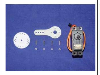
1. Turn on your transmitter and plug the servo into receiver. Ensure every channel is neutral
