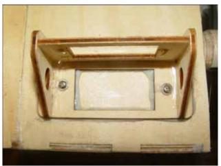
5. Finish the servo installation with mounting screws
