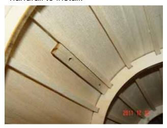
3. Cut the covering on the hole. Put some glue into the hole. Then put the handrail into the hole.
