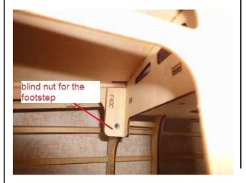
3. Put the footstep into the hole. Screw the bolt into the blind nut.
