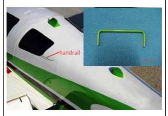
2. Find the reinforce wood for handrail which is inside of the fuselage. There are two holes for handrail to install.
