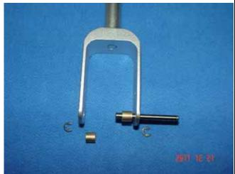
11. Install the tire into the front landing gear with the circlips outside.
