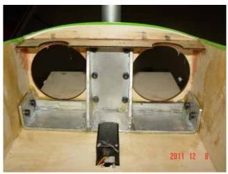
4 Outside view of mounting front landing gear.
