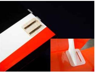
3. Scuff the middle of horns with a piece of sand paper for good glue bond. Then clean up the surface
