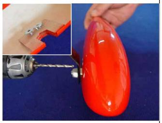
8. Finish the wheel pants mounting with the bolts.
