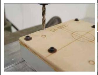
3. Drill the screw mounting holes aligning the line you have drawn both side as shown with the firewall taped or glued slightly in place(3mm bit)
