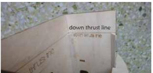
Note: The cowl is already pre-build for right thrust and down thrust. The center of the engine axle will be in the exact center of the cowl.
