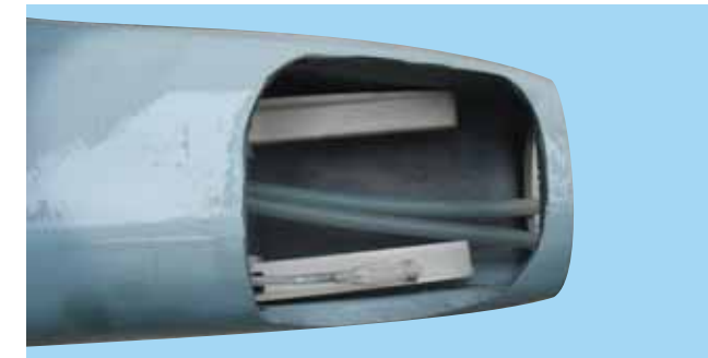
11C - Run external pressure, fuel and refuel lines through the firewall from the tank to the engine area
