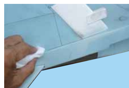
6F - Slide the vertical stabilizer into place. Wipe off any excess epoxy
