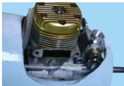
13A - Connect the clevis to the engine throttle arm
