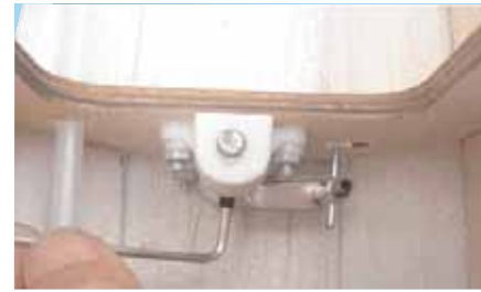
9G - After re-inserting the nose gear oleo strut, align and tighten the steering arm set screw.
