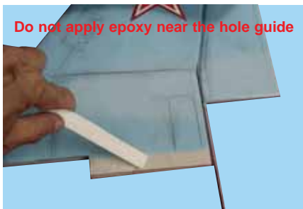
6D - Apply sufficient epoxy to both sides of the exposed wood
