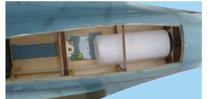
11B - Fuel tank assembly in position
