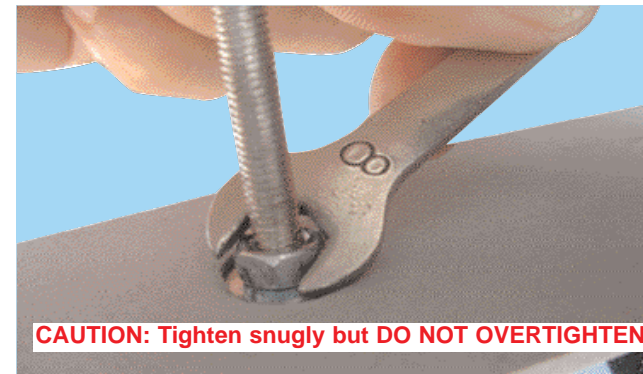
1H - Hold the wing bolt while tightening the lock nut
