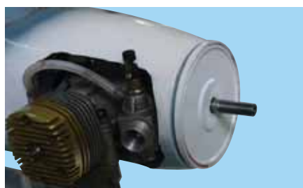
15B - Install the spinner backing plate
