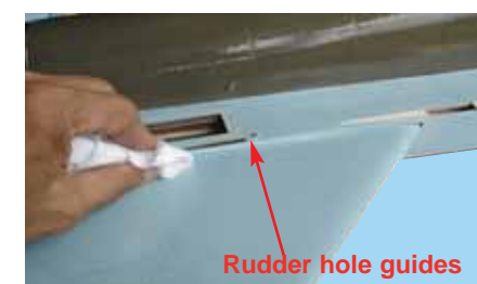
5E - Wipe off the excess epoxy to align the rudder hole guide
