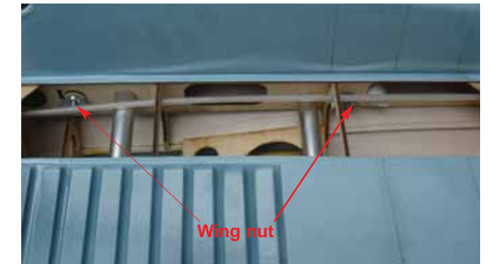
1K - Tighten the wing nuts. DO NOT OVERTIGHTEN. For double security also install the lock nuts
