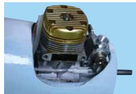
20A - The throttle arm and clevis connected to the engine throttle arm
