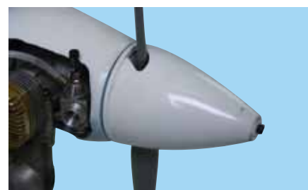
15D - Install the spinner cone using the retaining bolt. Ensure the retaining bolt is tight and secure
