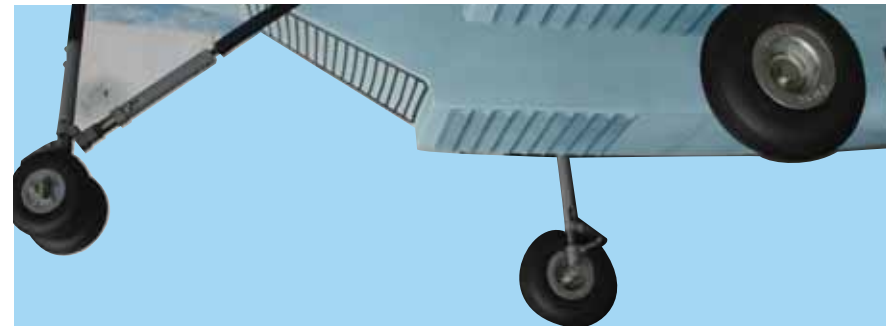
9I - Completed installation of the main and nose gear assemblies.
