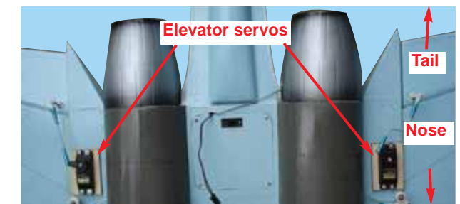
18B - Connecting the elevators to the servos
