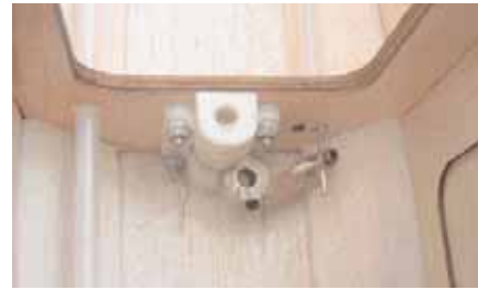
9F - Pass the nose gear steering rod through the EZ connector. Do not tighten yet.
