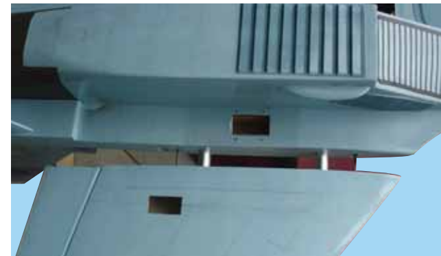
1J - Plug the wing panels into the fuselage
