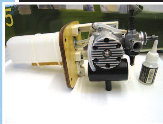
This is the power pod assembly with engine and fuel tank attached. Note my cable tie modification to secure the tank – more durable than the supplied rubber bands
