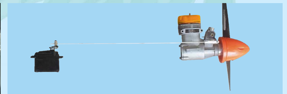
20B - The throttle servo controls the engine throttle using the throttle control rod
