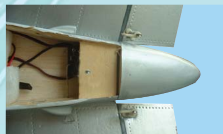
16C - Elevator control horns installed
