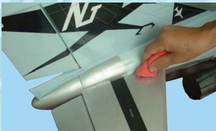
6E - Wipe off the excess epoxy
