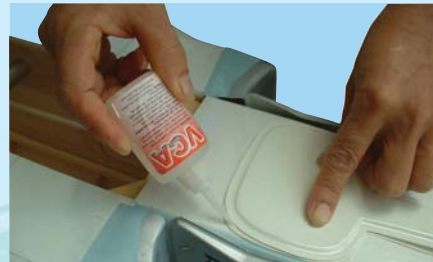
28C - Glue the nose gear cavity cover into place using CA glue
