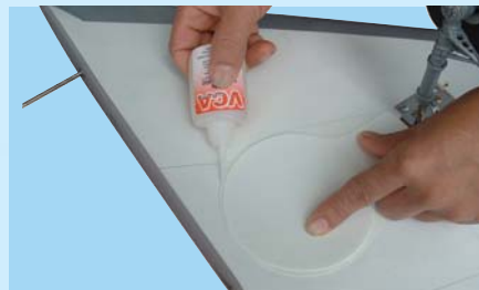
28B - Glue the main gear cavity covers into place using CA glue
