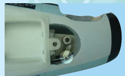
9B - Insert the nose gear push rod through the steering arm EZ-connector. Do not tighten yet
