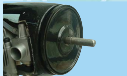
15B - Install the spinner backing plate
