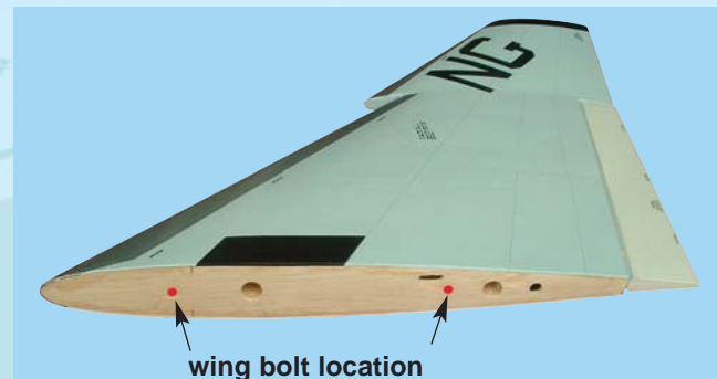
1E - The wing bolt location
