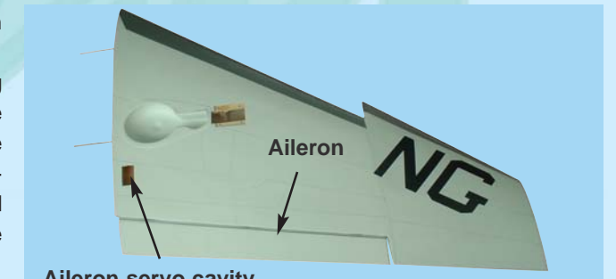
2B - Aileron servo location
