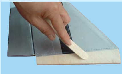
6C - Apply sufficient epoxy to the exposed wood area
