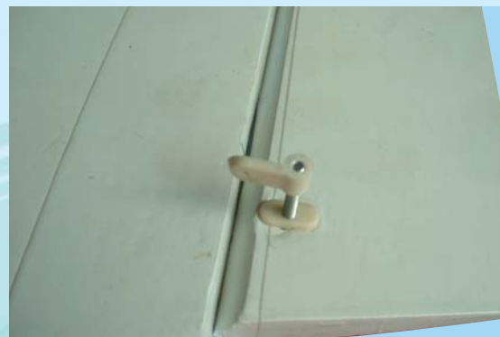
3B - Aileron control horn installed
