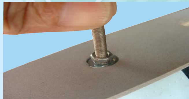
1F - Apply liquid thread locker and carefully thread the short end of the wing bolt into the hidden blind nuts in the wing
