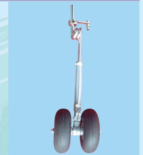
9A - Nose gear assembly
