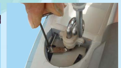
9D - Secure the EZ-connector to the nose gear push rod by tightening the set screw
