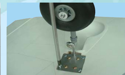
8C - Mounting the main landing gear to the wing
