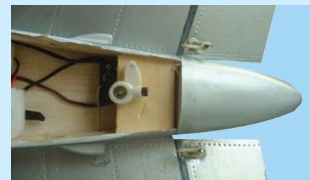
19C - Connect the clevis to the control horn and then tighten the set screw securely
