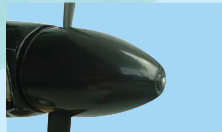
15D - Install the spinner cone using the retaining screw. Ensure the retaining screw is tight and secure
