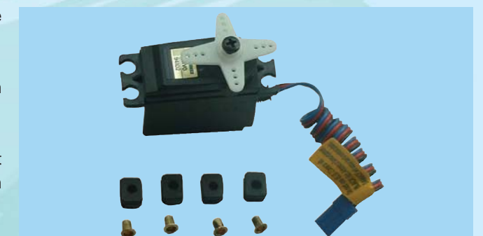
2A - Prepare the servos by fitting the rubber grommets & ferrules supplied with your servos
