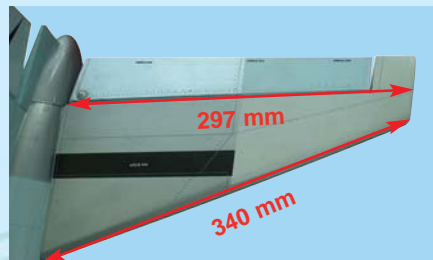
6D - Insert the left horizontal stabilizer into the fuselage and adjust the distance
