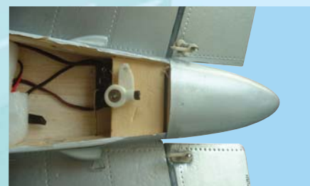
16D - Rudder control horn installed
