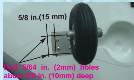
29B - Mark and drill mounting holes as indicated
