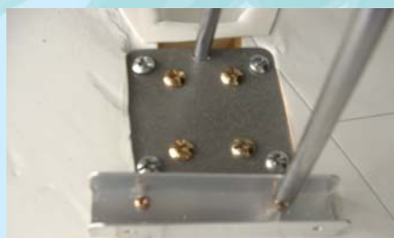
29C - Mount the dummy fuel tank to the wing
