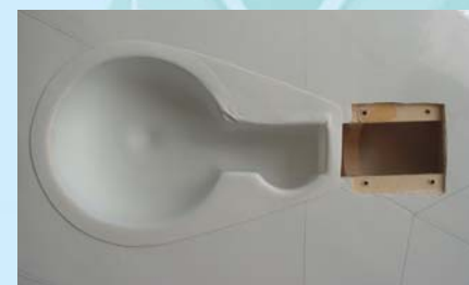
8B - Main landing gear location
