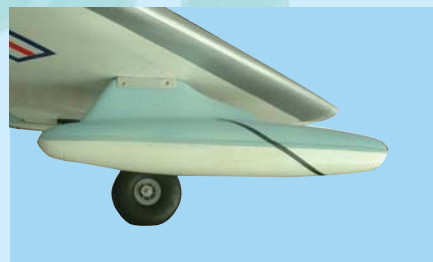
29D - Mount the dummy tanks to the aluminum racks on the wings
