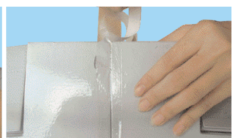
3C- Continue over the top of the wing and trim off the excess tape
