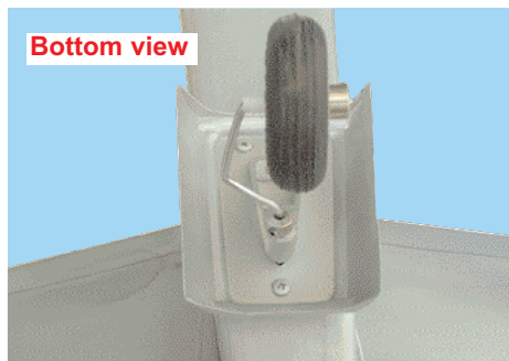
10A- Pre-installed tail wheel assembly with steering push rod
