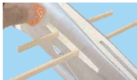
7B- Use CA glue to secure the horizontal joiner into the fuselage
