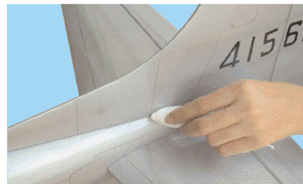
8E- Wipe off the excess epoxy
