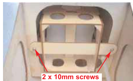
12C- Fuel tank assembly in position
