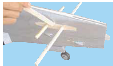
7E Apply sufficient 30 minute epoxy to the expose wood on the fuselage
