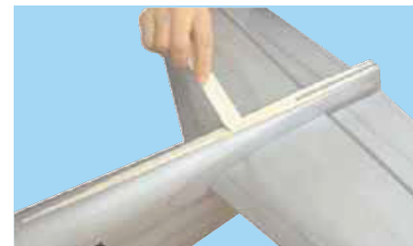
8C- Apply sufficient epoxy to the exposed wood area in the fuselage
