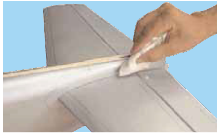
7H- Wipe off the excess epoxy
