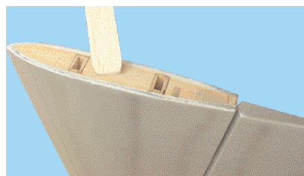
7D Apply sufficient 30 minute epoxy to the expose wood on both horizontal stabilizers
