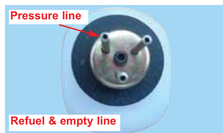
11B- Fuel tank and stopper assembly (front view)
