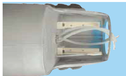
11D- Fuel tank installed into the fuselage after adding external fuel lines from tank forward to engine area
