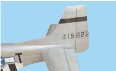
8A- Trial fit the vertical stabilizer into the fuselage
