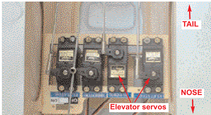
19A- Connecting the elevator control rod to the servos
