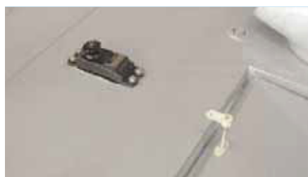
28B- Install the flap servos and flap control horns
