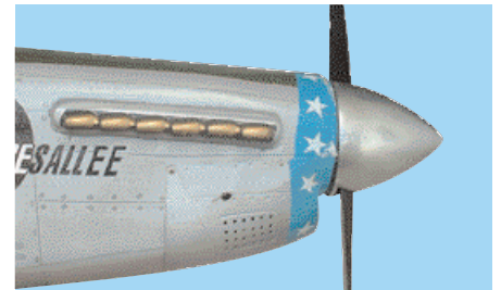
16D- Install the spinner cone using the retaining hex bolt. Ensure the retaining hex bolt is tight and secure
