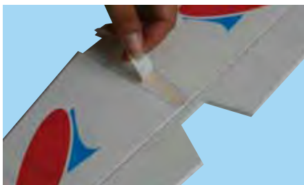
6E - Remove the covering from top surface
