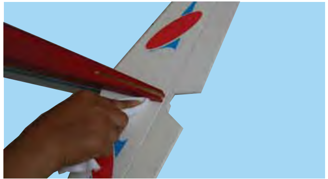
6K - Wipe off excess 30 minute epoxy
