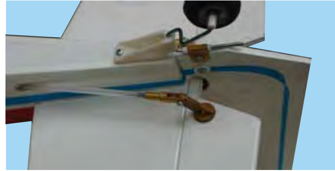
16B - Hold the elevator at neutral (not up, not down). Rotate the clevis to adjust the overall length. Then use the clevis screw to attach the clevis to the control horn. The clevis screw requires a 5/64 in. (2mm) hole. Secure the screw with thread lock
