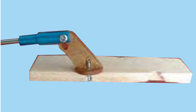
1A - Typical control horn installation.
