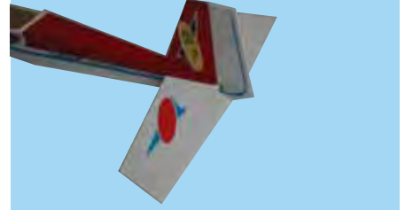
7A - Trial fit the vertical stabilizer into the fuselage slot
