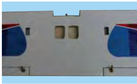
3B - Aileron control horn after installation.
