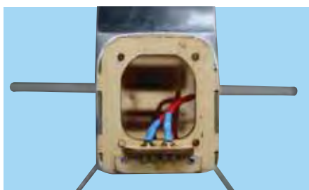
11H - Mount the pre-assembled fuse holder/switch to the fuselage by using two 2x8 [mm] screws
