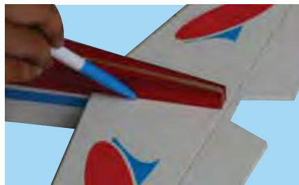
6A - Mark the top of the horizontal stabilizer...
