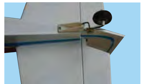
10D - Use two 2x10 [mm] screws to attach the tail wheel assembly to the fuselage.
