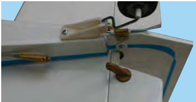
16A - Elevator control horn shown in position
