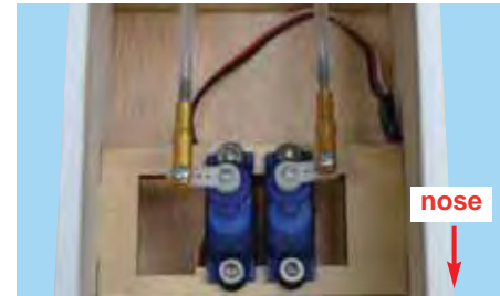
15A - Center the servos and control surfaces (rudder & elevator). Connect the control rods to the servos using the clevises as shown.
