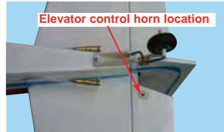
13C - Typical control horn location with respect to bottom of Elevator.
