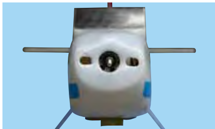
12B - Position the cowl over the mounting tabs. Align and center with respect to the motor shaft.
