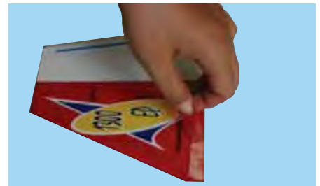
7D - Remove covering from both sides
