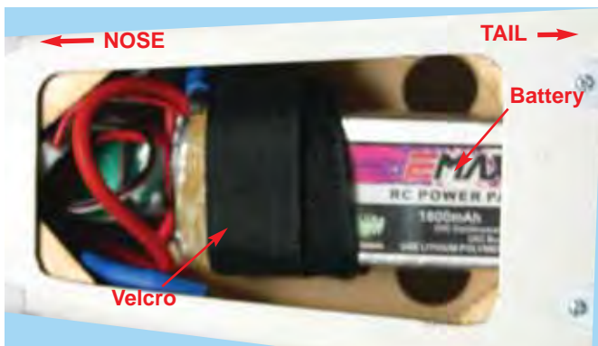
25C - Battery installed
