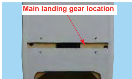
9B - Main landing gear location
