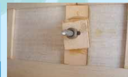
9D - Use the 4mm collar and set screw to secure the support strut.
