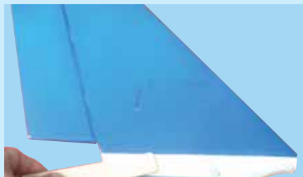
6C - Apply sufficient epoxy to the exposed wood area
