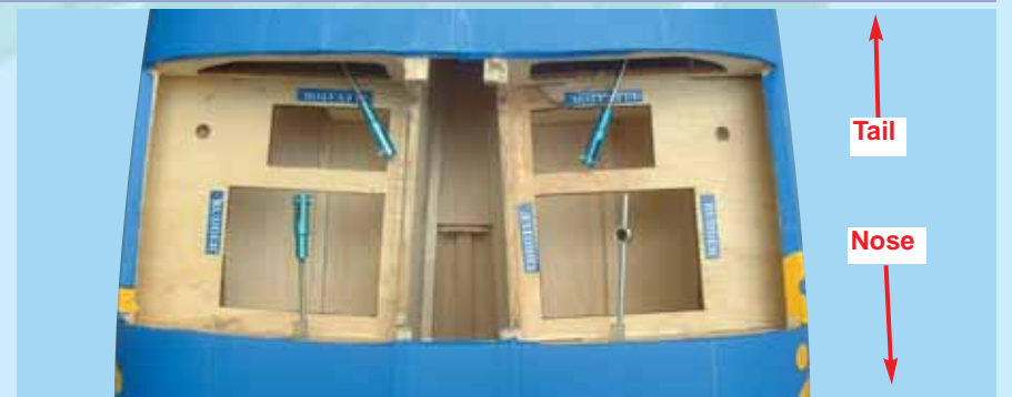
17A - Location of the 2 elevator, 2 rudder and throttle servos.
