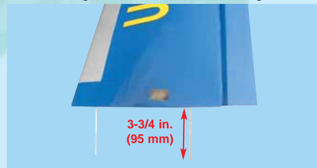
1G - Install the two wing bolts into the wing
