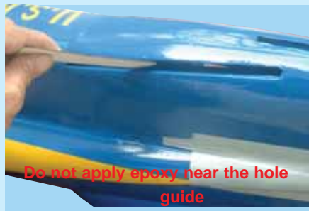
5D - Apply plenty of epoxy into the fuselage slot for the vertical stabilizer
