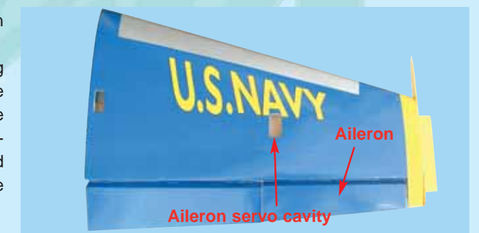
2B - Aileron servo location
