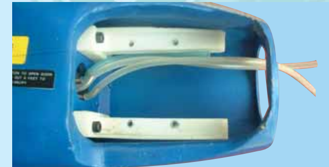
11C - Run external pressure, fuel and refuel lines through the firewall from the tank to the engine area
