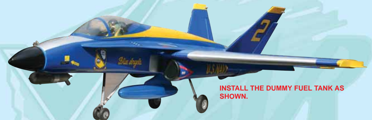
29C - Mount the dummy fuel tank to the hatch
