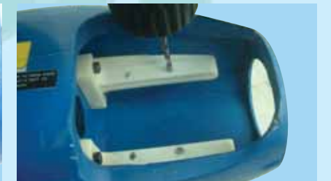
12D - Drill 3/32 in. (2 mm) pilot holes at right angles through the beams
