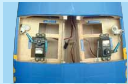
19C - With the servos and rudders at neutral, connect the clevises and then tighten the control horn set screws.
