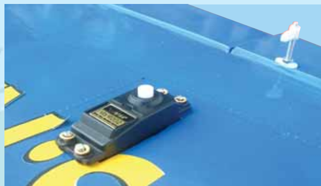
2C - Mount the aileron servos into the wing
