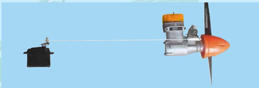
13B - Connect the servo arm to the engine throttle arm using the throttle control rod
