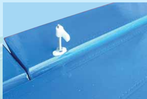
3B - Aileron control horn installed
