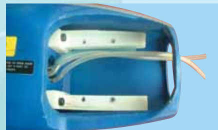
10D - Fuel tank installed into the fuselage after adding external fuel lines from tank forward to engine area
