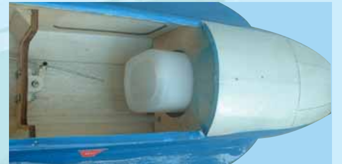
11B - Fuel tank assembly in position
