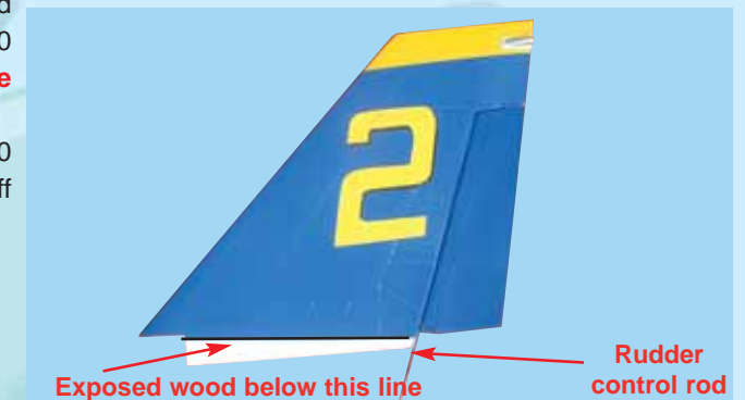
5A - Vertical stabilizer with pre-installed rudder and rudder control rod
