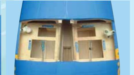
16D - Rudder control horns installed
