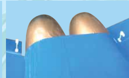
16C - Elevator control horns installed
