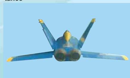
6F - Vertical and horizontal stabilizers installed.
