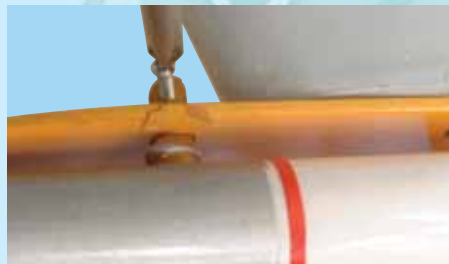
30D- Secure the front end of the missile
