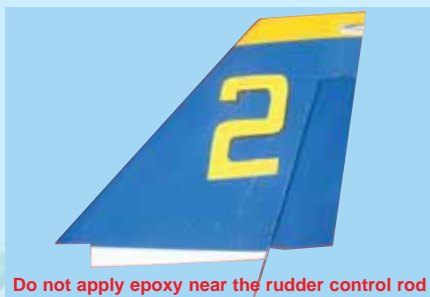
5E - Apply sufficient epoxy to both sides of the exposed wood
