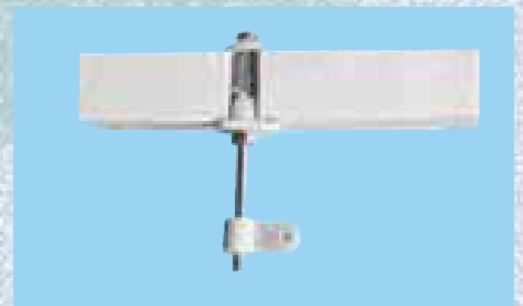
21B - Typical control horn mounted to a control surface
