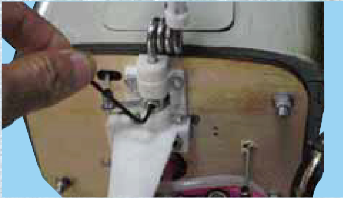
15E - Insert the nose gear into the bearing, passing through the steering arm. Secure the steering arm to the nose gear by tightening the set screw onto the flat spot on the nose gear wire
