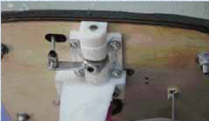
15C - Turn the fuselage upside down and insert the end of the pre-installed nose gear steering wire into the EZ connector pre-installed to the steering arm
