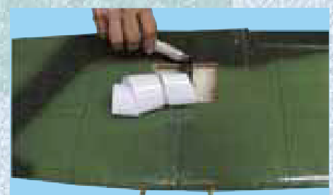
3C- Continue over to the bottom of the wing & along to the servo cavity and trim off the excess tape
