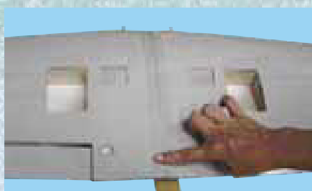
3B- Continue applying the tape over the top of the wing, pressing down firmly as you go
