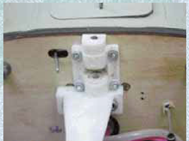
15B - Install the nose gear bearing to the power module
