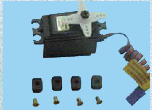
4A - Prepare the servo by fitting the rubber grommets & ferrules supplied with your radio
