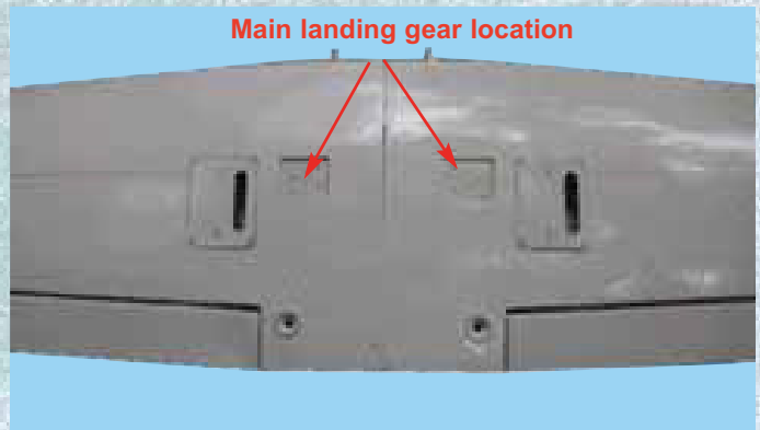
14B - Main landing gear location located under the wing
