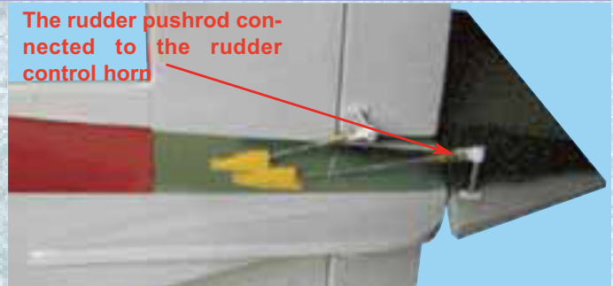
25A - The rudder pushrod connected to the rudder control horn
