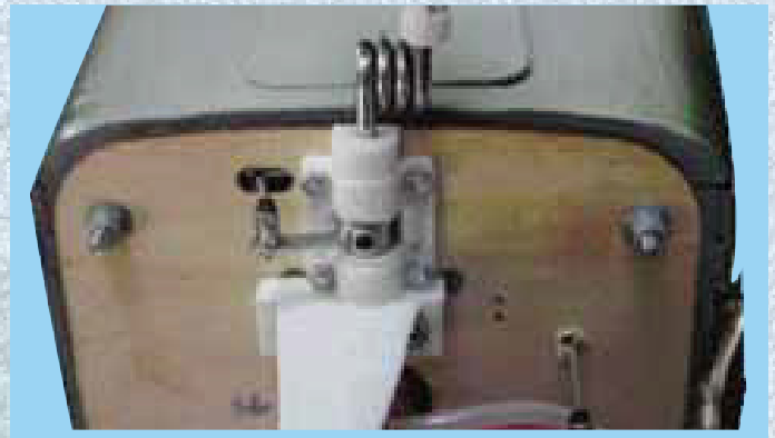
15D - Place the steering arm into the slot in the nylon nose gear bearing
