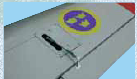
5C - Aileron servo and control rods installed
