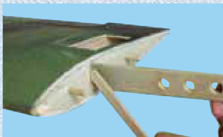
2A - Apply plenty of 30 minute epoxy glue to all surfaces
