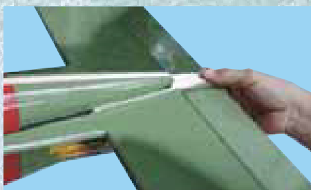
10C - Slide the horizontal stabilizer in place
