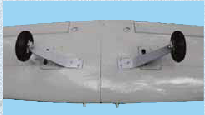
14D - Right and left main landing gear mount to the wing
