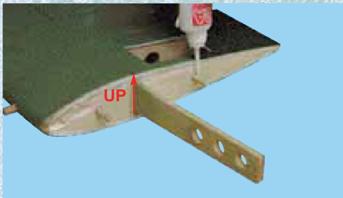
1C - Apply CA glue to secure dowels into their places
