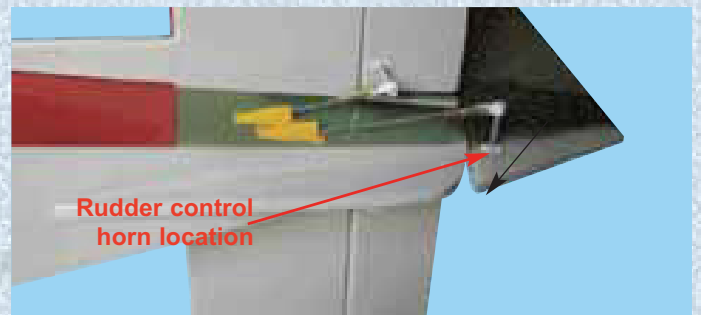
21D - Rudder control horn location
