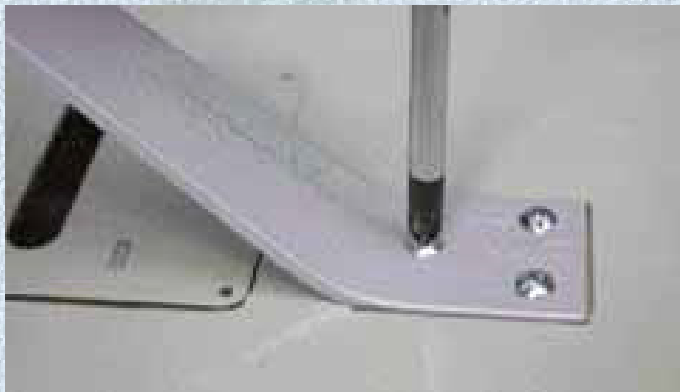
14C - Use three 3 x 15mm screws to mount the main landing gear to the wing
