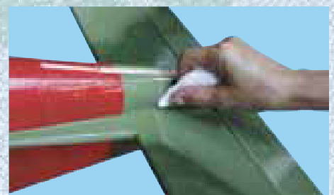
10D - Wipe off excess epoxy
