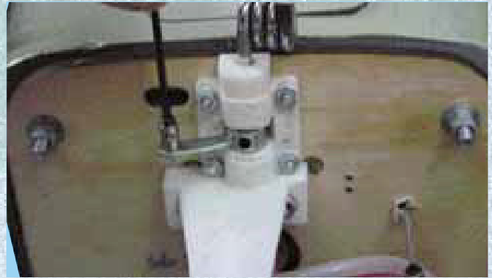
15F - Then tightening the set steering arm to the nose gear control rod
