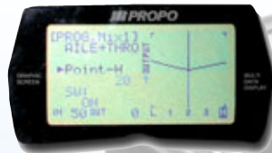
Aileron to Throttle mixing on X-3810
