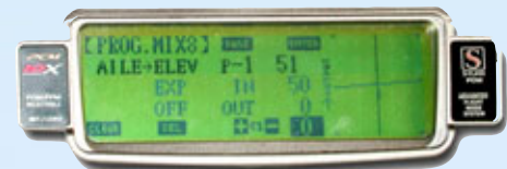
Manual Swashplate Timing with PCM10x
